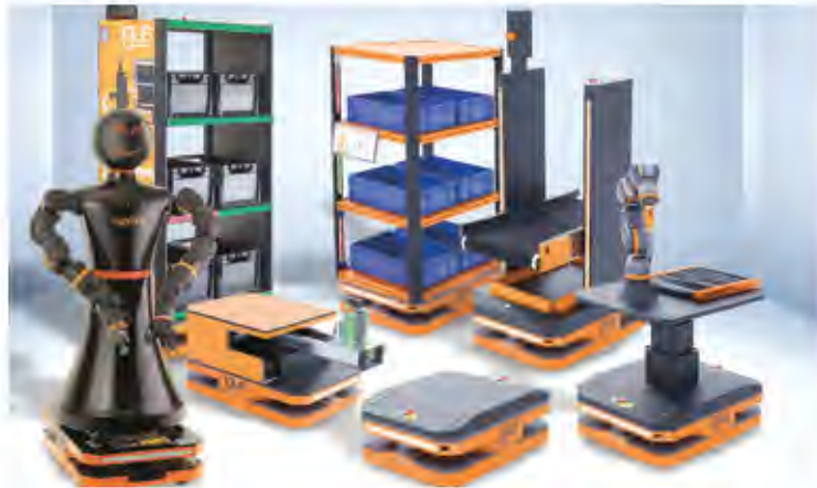
The ReBeLMove Pro serves as a platform for various superstructures, from order-picking systems to intelligent shelving systems to collaborative robots with conveyor belts. (Source: igus GmbH)
